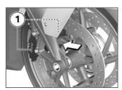
Visually inspect the left and right brake pads to ascertain their thickness. Direction of view: between wheel and front wheel control to brake calipers 1.
